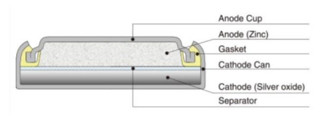
Watch battery maker Murata has announced that it has produced over 4 billion units of no-mercury, silver-oxide micro-batteries, saving 7,055 pounds (3,200 kg) of mercury from potentially entering into the environment from spent batteries.
